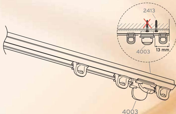
Tracks can be slotted for ease of adding extra gliders.
